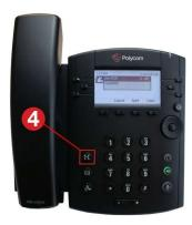
Press the Transfer button again to complete the transfer. The
